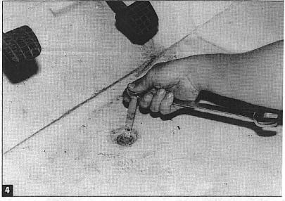
When the truck is high enough for adequate access to the mounts, loosen each of the bull but do not remove them. You may have to use some of your favorite rust buster to get the factory nuts loose. Only loosen one side at a time. Keep in mind you may have to remove your carpeting to access the head of the mount bolts.
