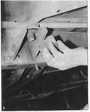
When the bolts are removed from one side, go ahead and remove the lower rubber mount, as shown.
